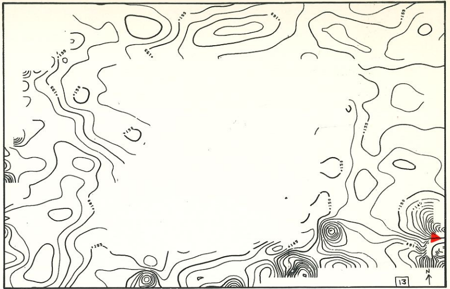
Figure 7. Contour map of magnetic intensity over Monument 61 (shown in Figure 6). The head was found under the anomalous area indicated by the colored marker in the
