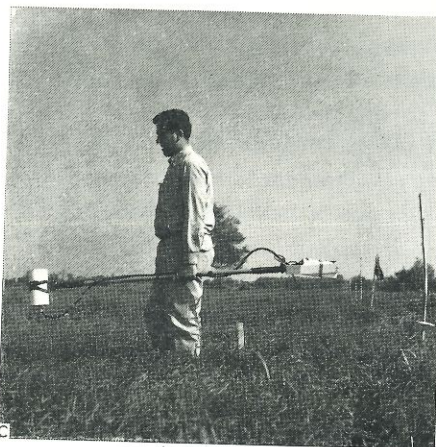
Fig.4A. Block diagrams of two configurations for the fixed and mobile magnetometer stations for difference mode of operation. B. Digital readout unit (weight 8 lb.). C. Mobile sensor (weight 6 lb.). Fixed sensor (not shown) identical. Battery pack (not shown) weight 15 lb.
