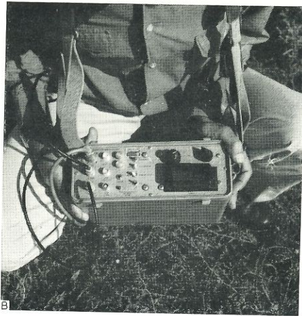
Fig.4A. Block diagrams of two configurations for the fixed and mobile magnetometer stations for difference mode of operation. B. Digital readout unit (weight 8 lb.). C. Mobile sensor (weight 6 lb.). Fixed sensor (not shown) identical. Battery pack (not shown) weight 15 lb.
