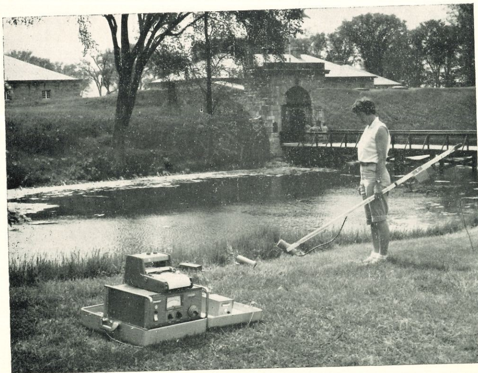
PLATE 1. Complete assembly of rubidium magnetometer and sensors (one held by E. K. Ralph) at Fort Lennox, Ile-aux-Noix, Quebec P., Canada, May 1964. (Power cable leading to the fort is not shown.)
