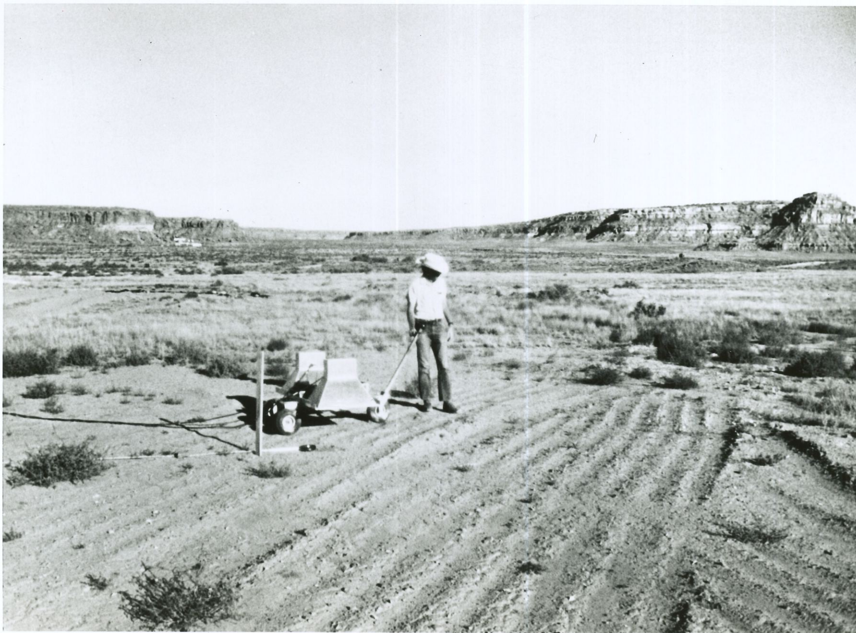
FIGURE 2 CHACO CANYON ANTENNAS ON HAND CART
