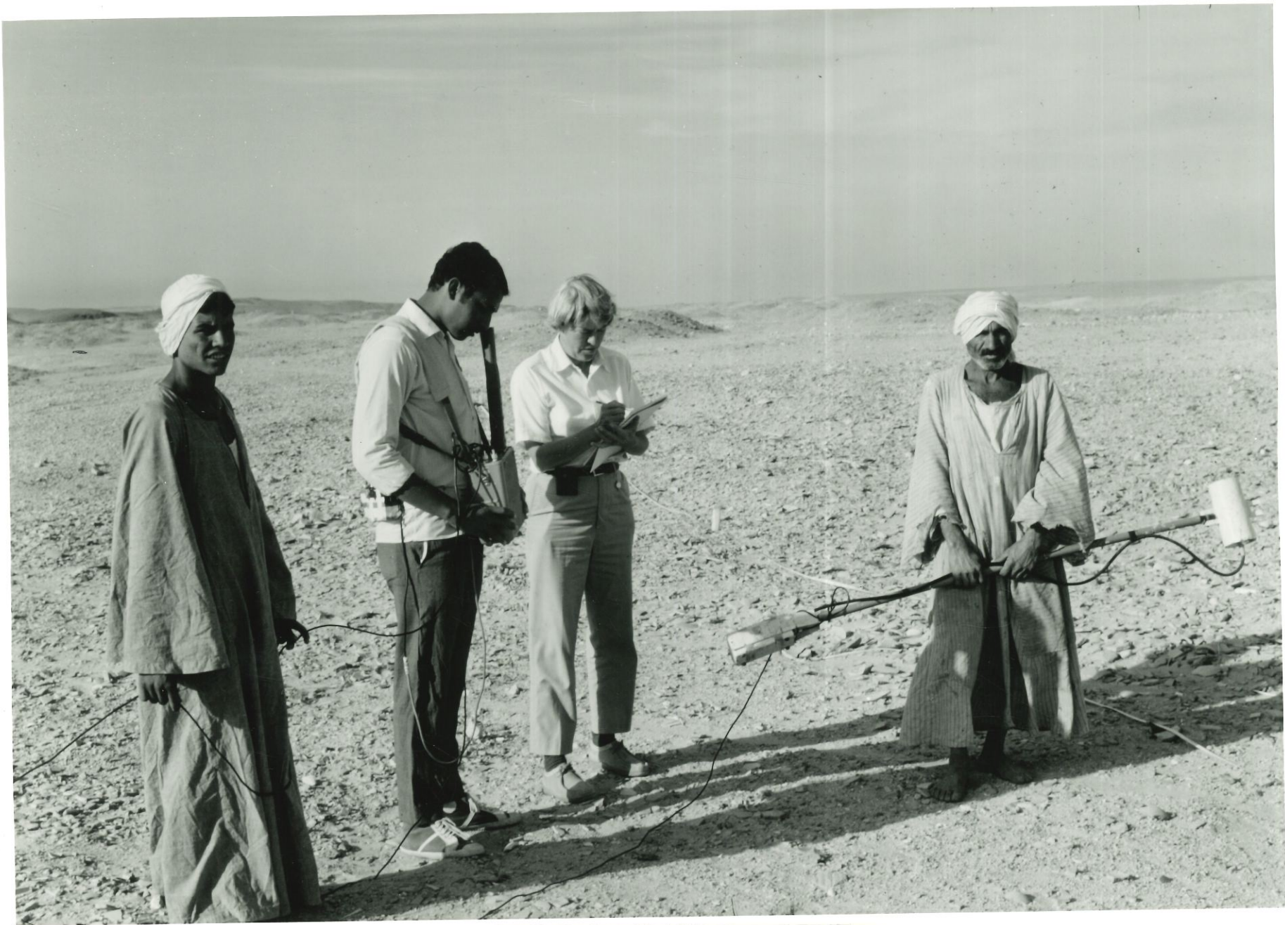
Fig. 2 Cesium Magnetometer and Crew at Malkata. Left to right: Hamedy with cable, Badauy with readout, Beth with notebook, and Zakhry with sensor.
