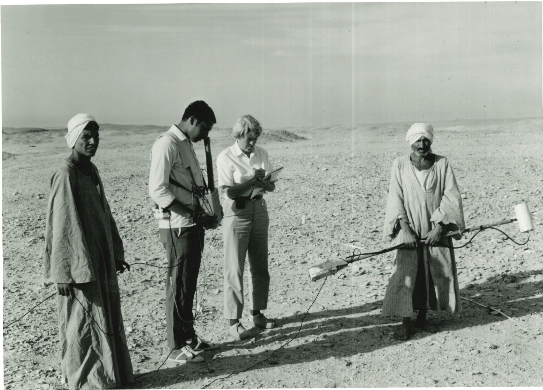
Fig. 2 Cesium Magnetometer and Crew at Malkata. Left to right: Hamedy with cable, Badauy with readout, Beth with notebook, and Zahkry with sensor.
