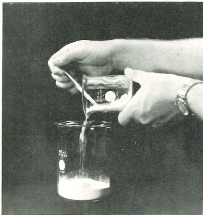
Slight wetting (or swelling) results when water is poured on VOLCLAY.
